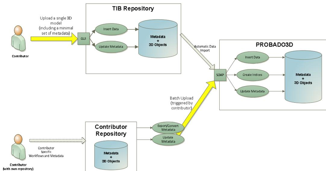
Figure 1. Use-case for integrating 3D models into PROBADO3D
